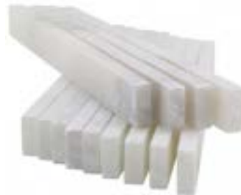
Flat Soapstone Item PWDFS1 • 5 L x 1/2 W x 3/16 H" • Temporary marking of metal for welds • Easily removable • Will not contaminate welds • 144/Box
