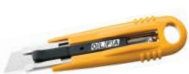
Semi-Automatic Self-Retracting Safety Knife Item OLFSK4 (19 mm) • Spring-activated blade retracts when lifted from cutting surface • Stainless steel return spring and channel • Dual-edge safety blade
