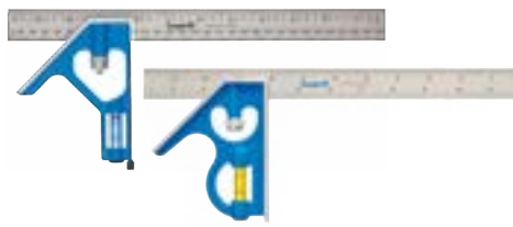
Combination Square Item EMP240IM Item EMPE250IM (w/ scribe pin) • Etched stainless steel blade • Full view acrylic vial • Self-aligning drawbolt • 11.8" with SAE/metric graduations
