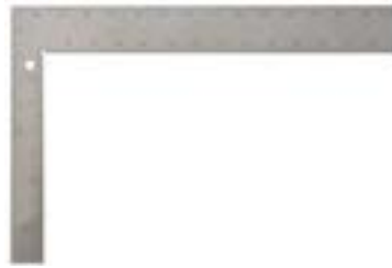
Steel Square Item EMP100IM (12 x 8 in) Item EMP1110IM (24 x 16 in) • Alloy steel • Stamped numbers • 1/8" graduation • SAE/metric units
